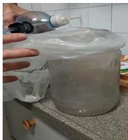
Fig. 2 Approximately 10 seconds after the introduction of Sunny Rain condensation nuclei: the visible smoke had dissipated and condensed water had accumulated on the inner walls of the container.
