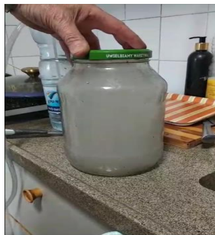
Fig. 1 Airtight container filled with dense smoke produced by waste incineration before the introduction of Sunny Rain condensation nuclei.
