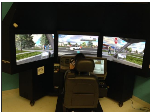
Fig. 1 TranSim VS IV driving simulator employed in the experiment.
