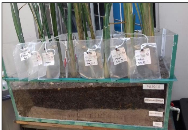
Fig. 7 Wetland with methane collection tube system and sampling bags.
