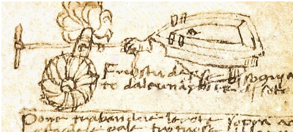
Figure 5. Human-powered system for imparting to pull a vessel in water. Opusculum de architectura . Francesco di Giorgio (Detail). Biblioteca Apostolica Vaticana. Rome. Italy.
