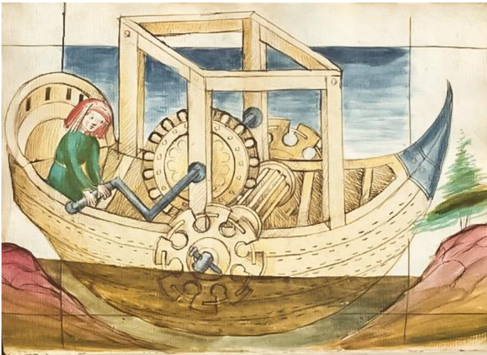
Figure 3. Human-powered paddle-wheel vessel as depicted in the Frankfurt manuscript of Bellifortis by Konrad Kyeser 5 . 1460. Universitätsbibliothek Frankfurt am Main. Ms. germ. qu. 15 (Detail).
