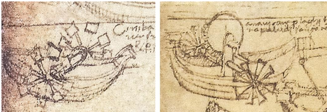
Figure 7. Projects of small wheel boats from the Taccuino of Francesco di Giorgio. Left, Folio 18; right Folio 19v (Details). Biblioteca Apostolica Vaticana. Rome. Italy.
