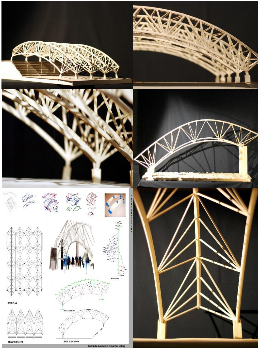
Fig. 9 Design projects by students. Community hall structure. The student team designed a module of a curved, folded-plate truss, repeating over 4 bays. Anticipating more compressive stresses on the top chord, and more tension along the bottom chord, diagonals were laid out to have more joints along the top, resulting in shorter length top-chord bars and longer length bottom-chord tension rods. Graphic analyses at bottom left.
