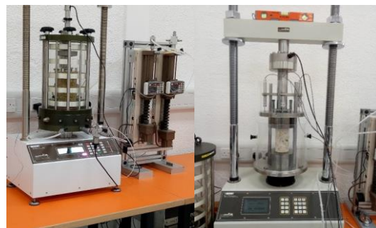
Fig. 16 Photos of UCS and CIU tri-axial computer controlled testing machines (GTC-LAB, 2017).
