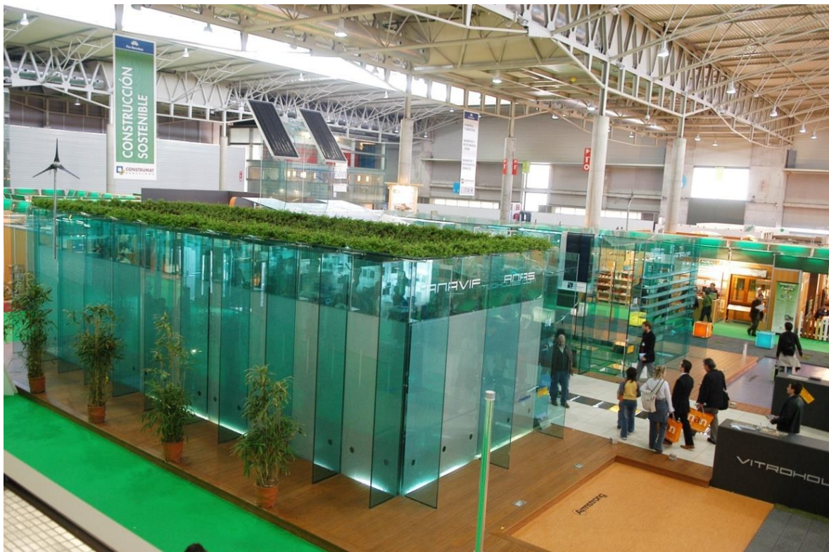
Fig. 8 The left side of Vitrohouse incorporates glass whose opacity changes through small electric currents, regulating privacy and solar protection.
