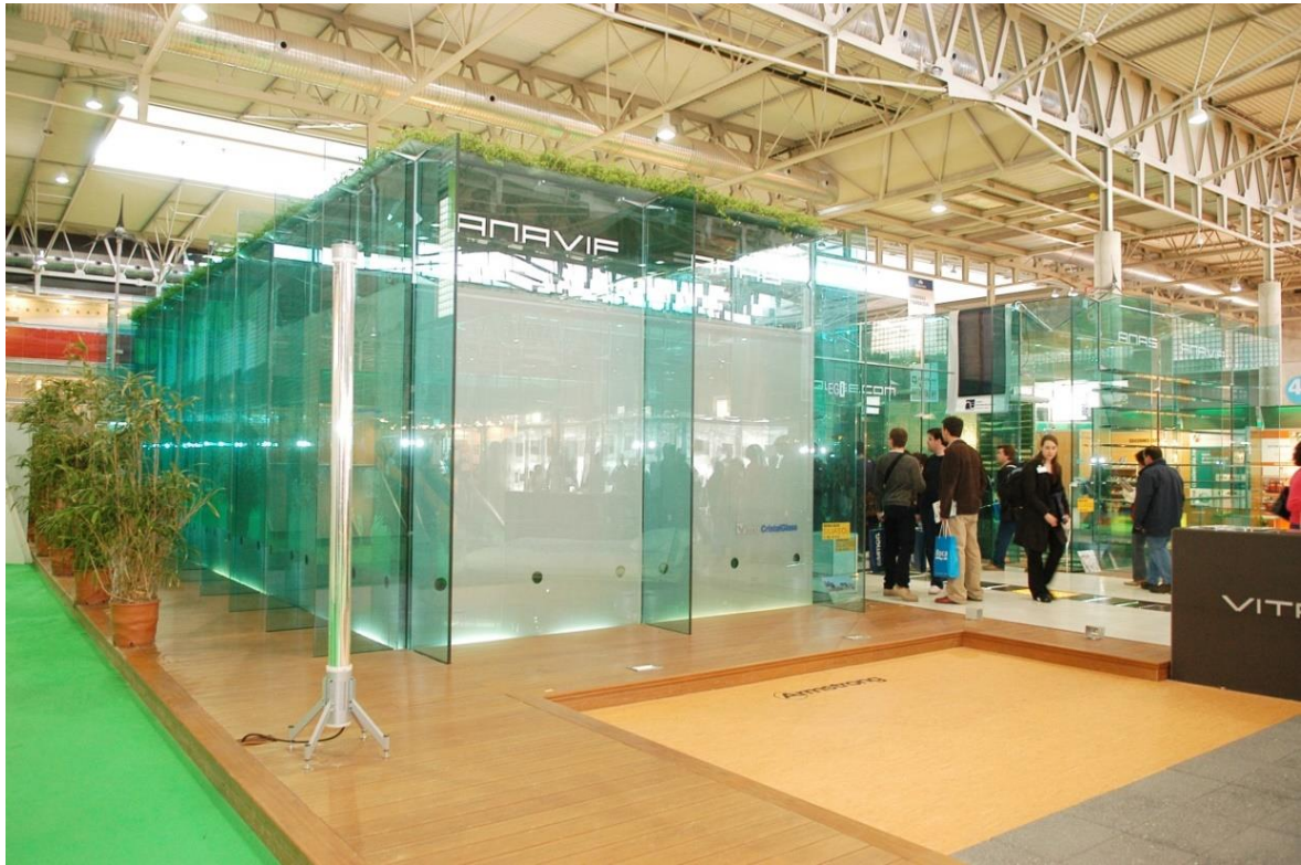
Fig. 7 Vitrohouse's architectural envelopes are highly varied and include a triple glass skin with two air chambers: a sealed inner chamber and a ventilated outer chamber. The outer chamber includes blinds that regulate sunlight from zero to 100%.
