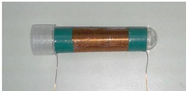
Fig. 3 Solenoid built to perform the measurements.
