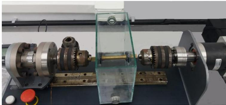
**Fig. 7** Torque measurement bench.
