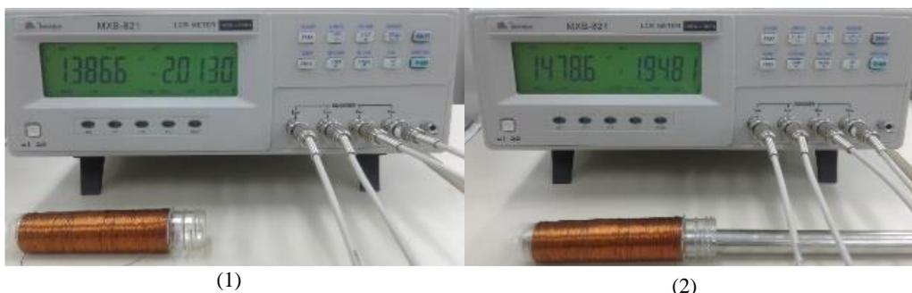
Fig. 4 RLC bridge for measurements.
