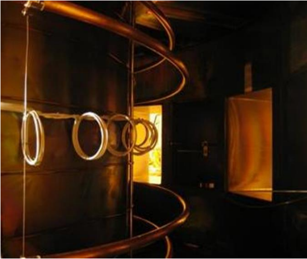
Fig. 12 The solenoid used to enhance the toroidal magnetic field.
