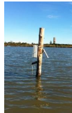
Fig. 8 Data logger located in a HCW ("Valle da Pesca").
