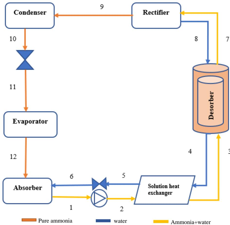
Fig. 1 Ammonia-water absorption machine.
