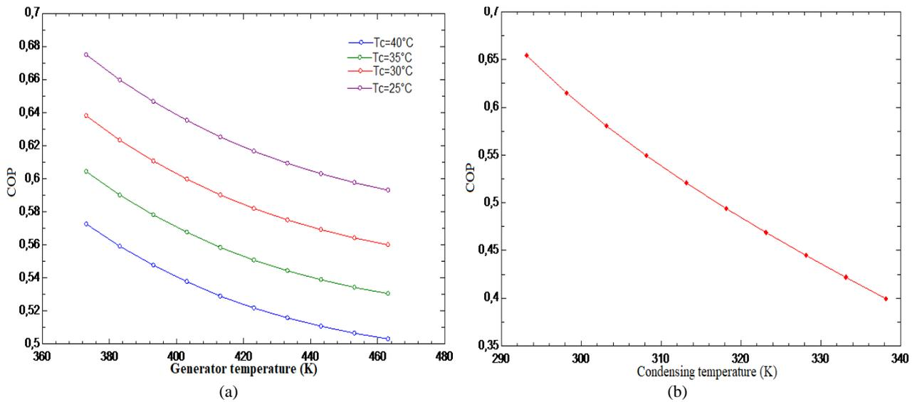
Fig. 4 (a) COP variation as a function of generator temperature for different condensing temperatures; (b) COP variation as a function of condensing temperature.
