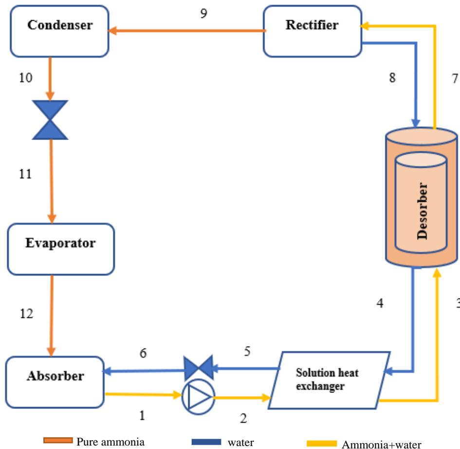
Fig. 1 Ammonia-water absorption machine.
