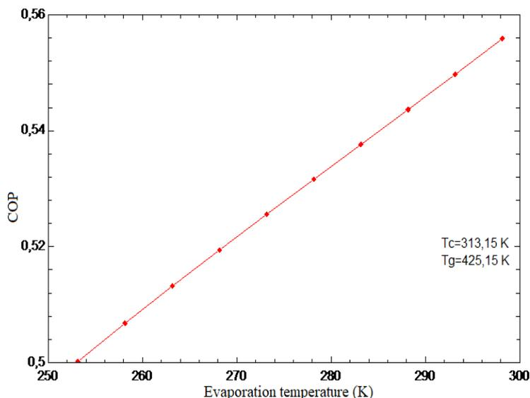
**Fig. 5** Variation of COP with evaporating temperature.
