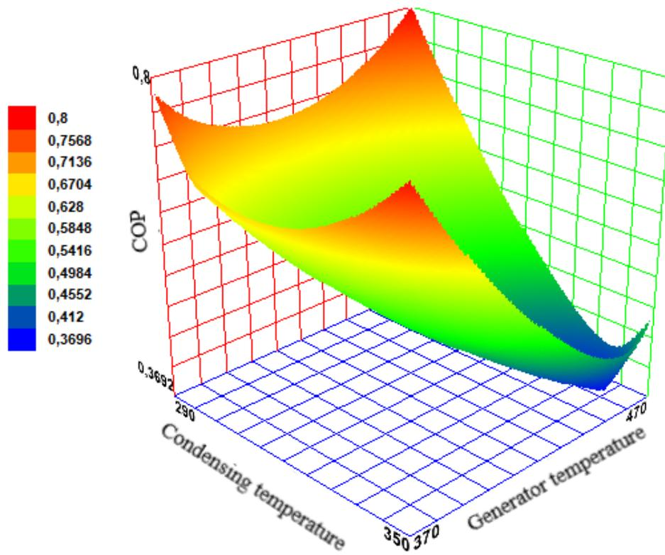
Fig. 3 COP variation as a function of generator temperature and condensation temperature.
