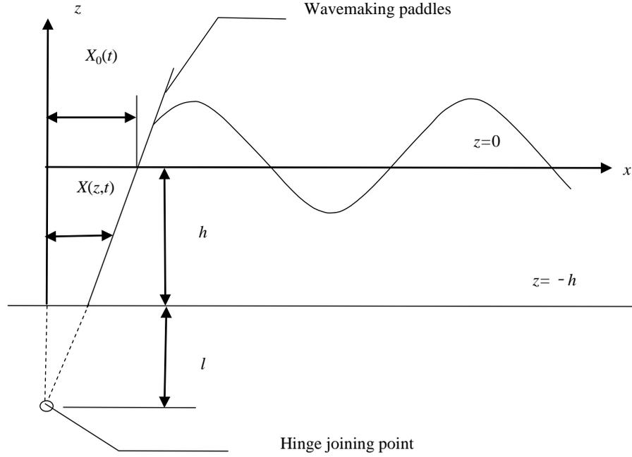
**Fig. 2 Wave-maker geometry and definition of notation.**
