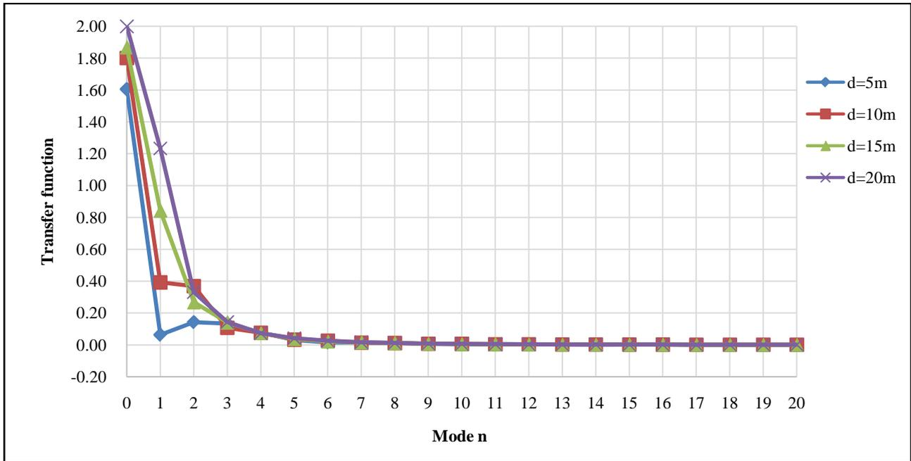
**Fig. 5** The change curve of transfer function with order at different hinge depth.
