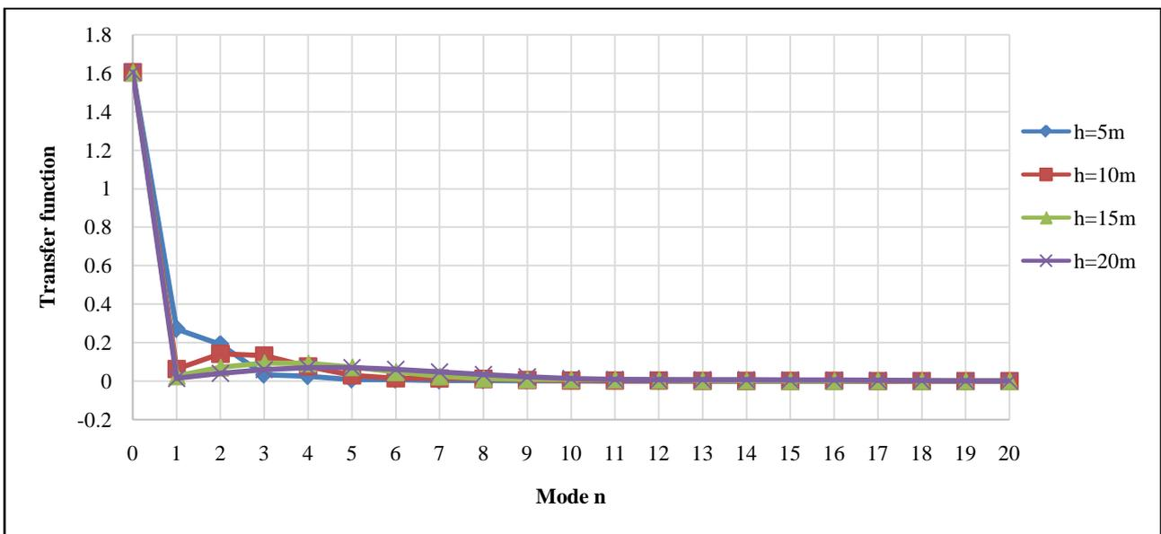
Fig. 4 The change curve of transfer function with order at different water depths.
