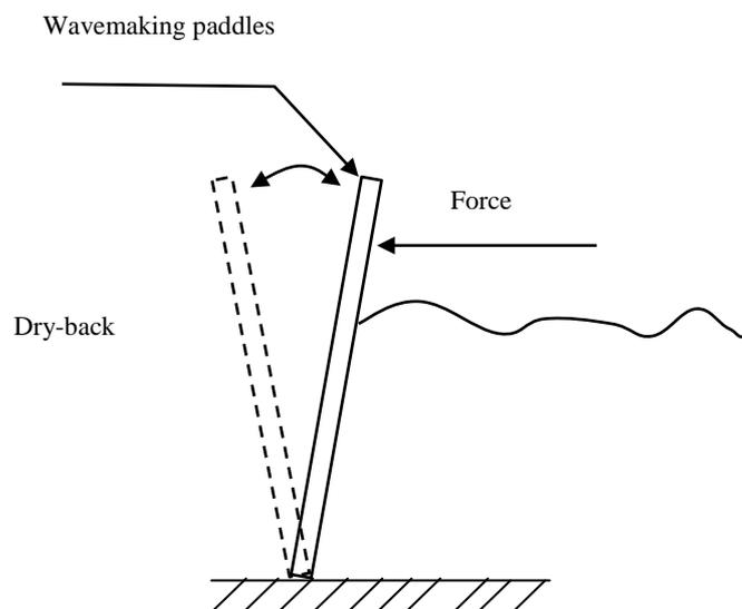
**Fig. 1** Layout diagram of force-feedback active absorption test.
