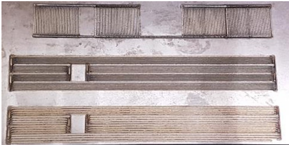
Fig. 6 250 W at 25 mm/s laser build on flat 10 mm thick plate with SG spaces.
