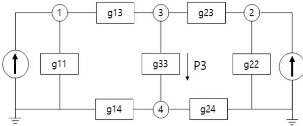
Fig. 7 Equivalent circuit of DC urban railway system.
