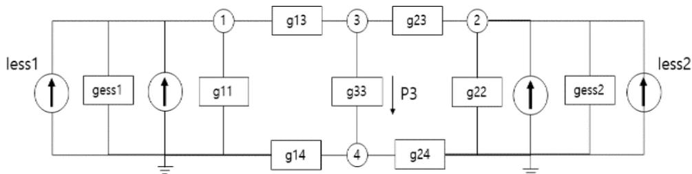
Fig. 9 Equivalent circuitry for railway systems with ESS installed.
