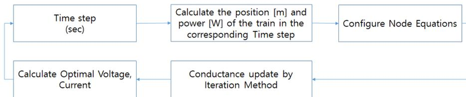
Fig. 3 DC feeding power simulation algorithm.
