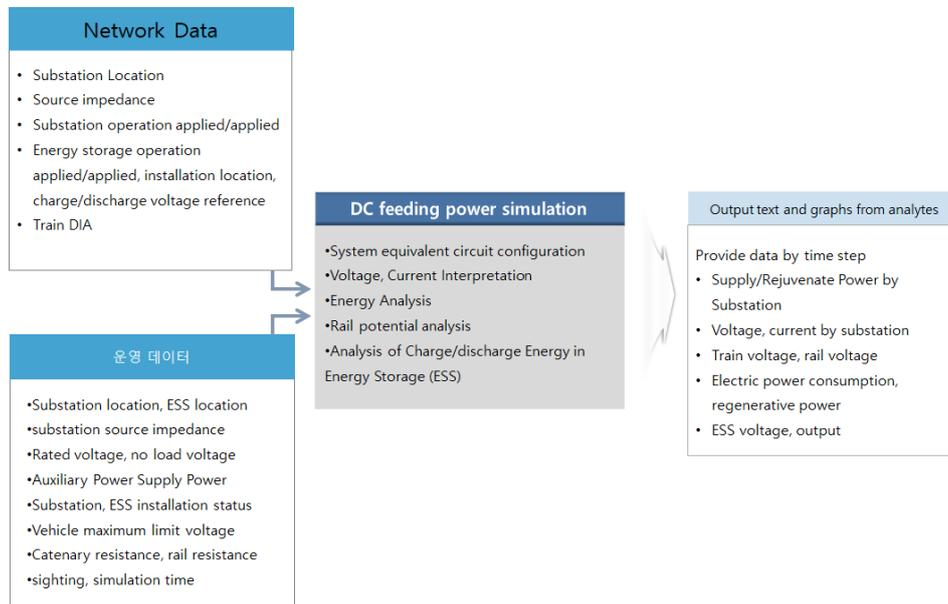
Fig. 2 Key features of DC feeding power simulation.
