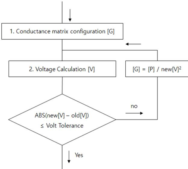
Fig. 8 Algorithm for load flow calculation by conductance matrix repeating method.
