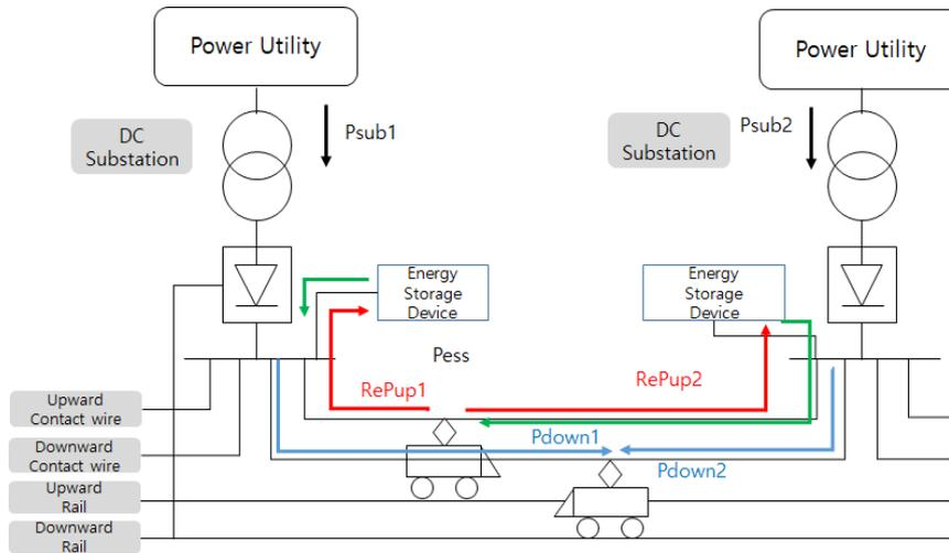
Fig. 4 Flow chart of the DC electric railway system.
