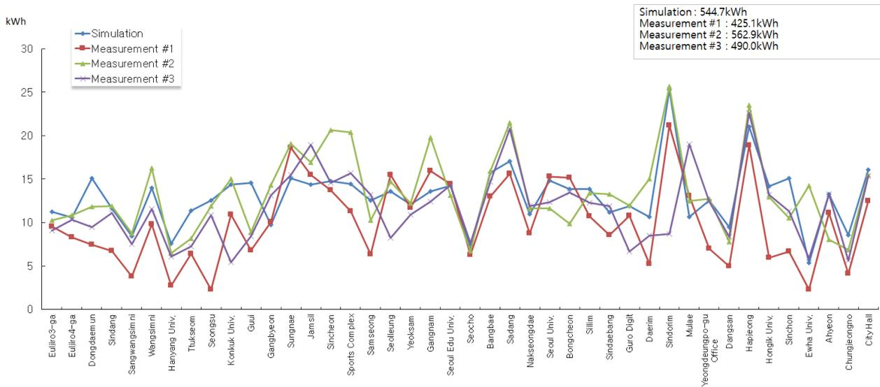
**Fig. 12 Regenerative energy(measurement & simulation).**
