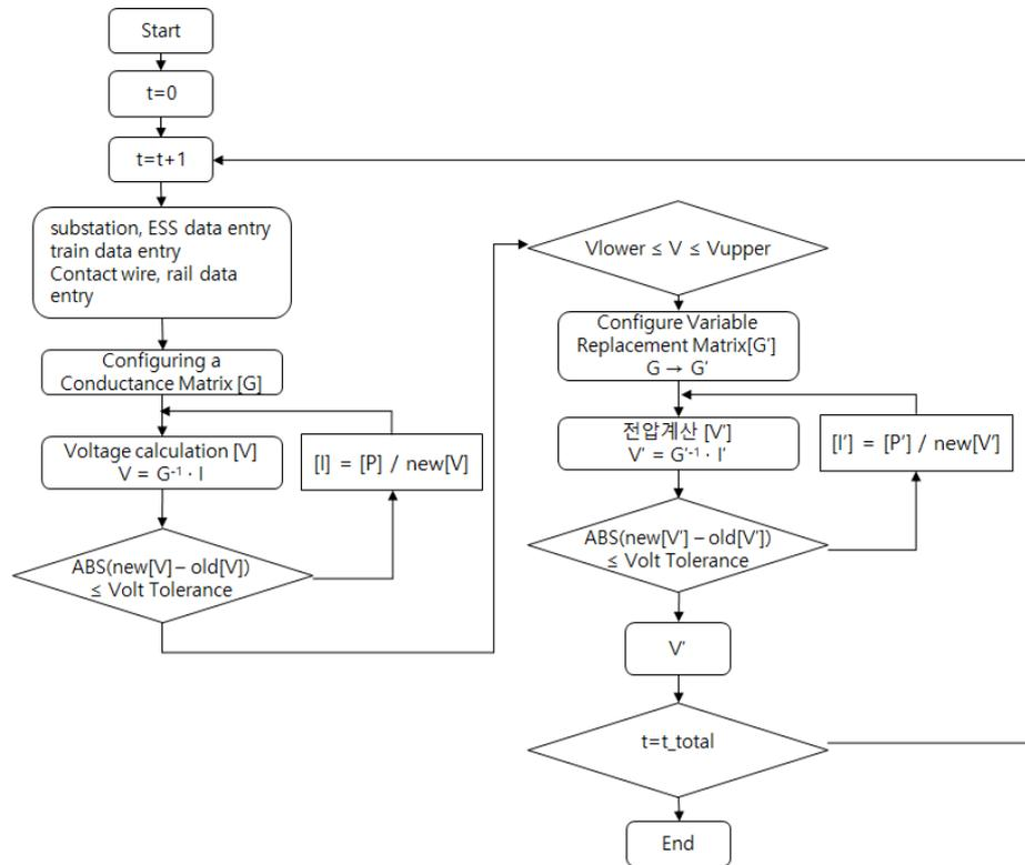
Fig. 10 ESS voltage control range optimization algorithm.
