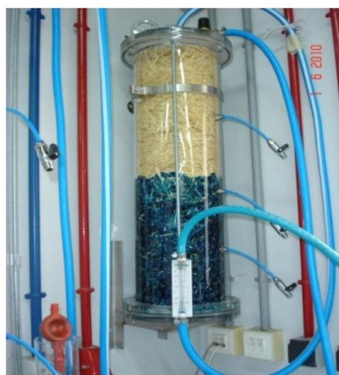
Fig. 1 Bed length adsorption column 75 cm from plexiglass with adsorbent material of chickpea straw and adsorbable substance methylene blue.
