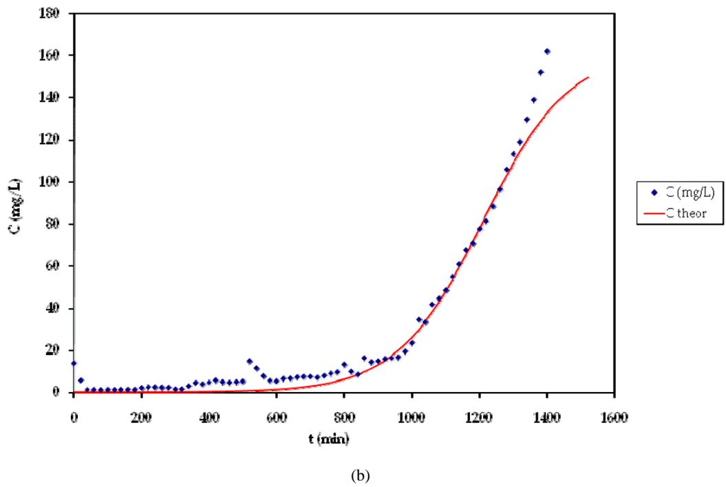
Fig. 5 Experimental and theoretical points of the sigmoidal adsorption curve as a function (a) of volume and (b) of time in a 75 cm long column.
