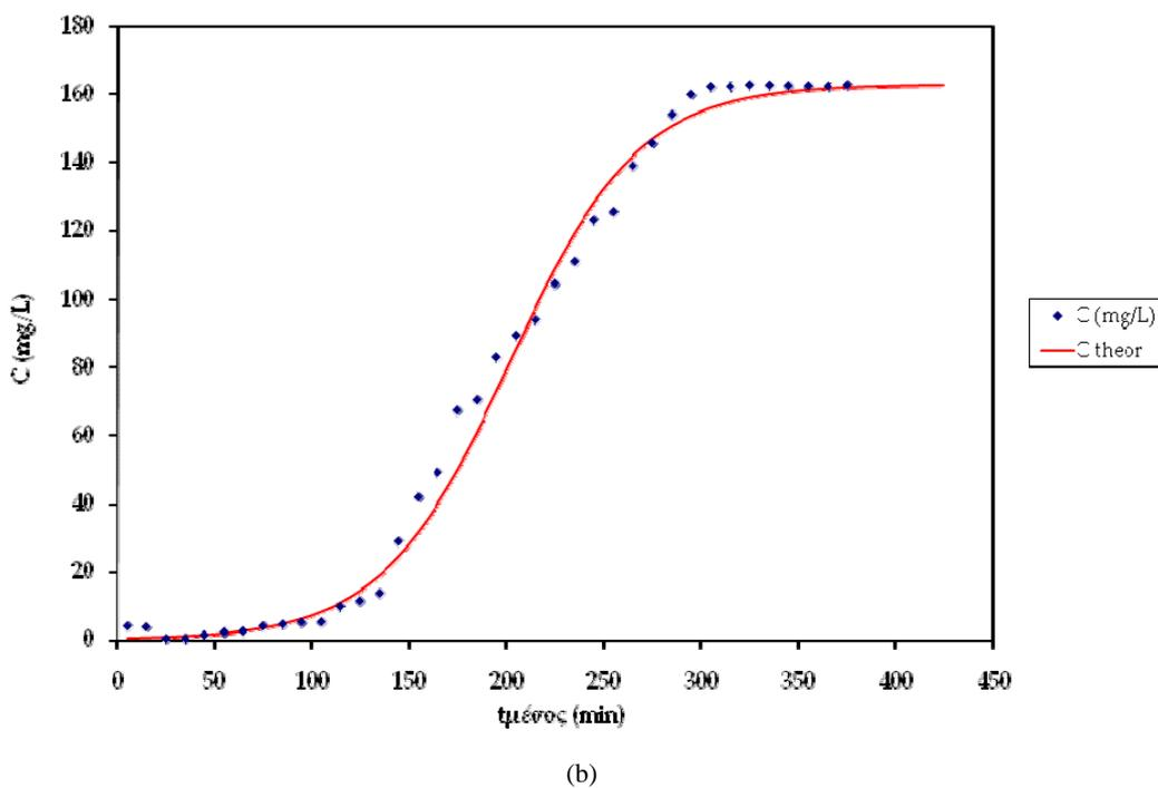
Fig. 4 Experimental and theoretical points of the sigmoid absorption curve as a function (a) of volume and (b) of time in a 25 cm long column.
