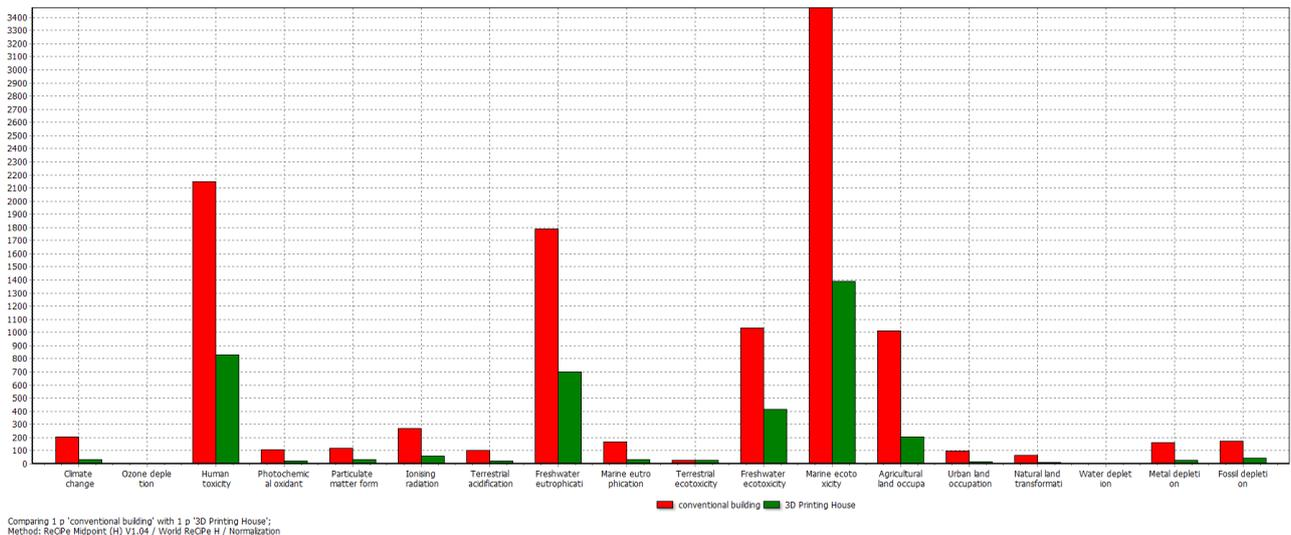
Fig. 6 Normalization results of the two alternatives using ReCipe midpoint.
