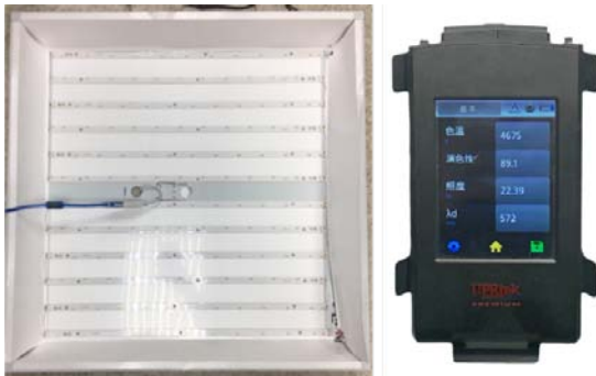
Fig. 18 Dimming measurement result of brightness level 0 (0%).
