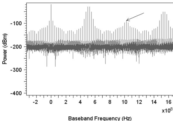
Fig. 2 RF Spectra of two tone directly modulated, CSO distortion at 1025 MHz.
