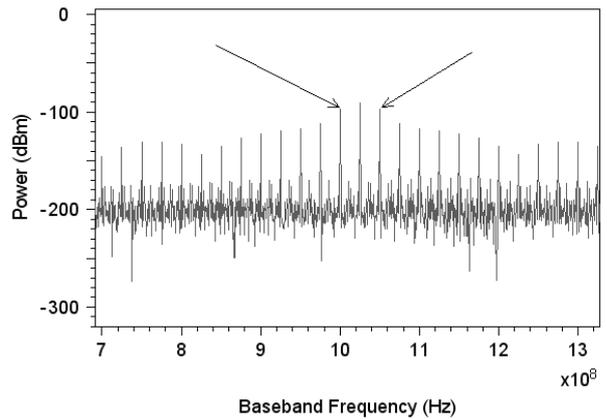
Fig. 3 RF Spectra of two tone directly modulated; IMD at 1000 MHz & 1050 MHz.
