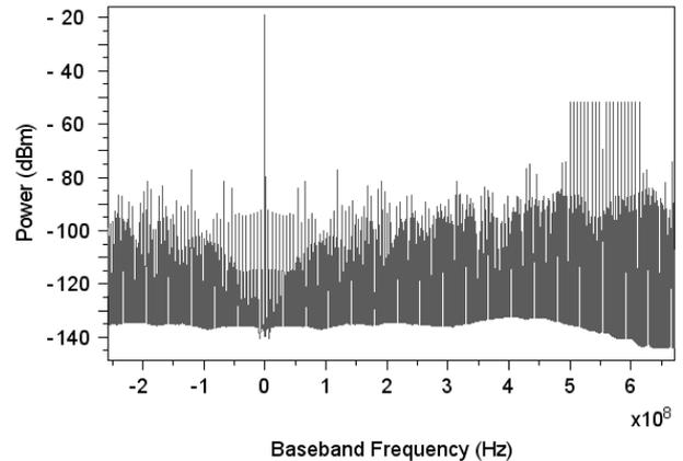
Fig. 7 RF Spectra of to 20 channel directly modulated.
