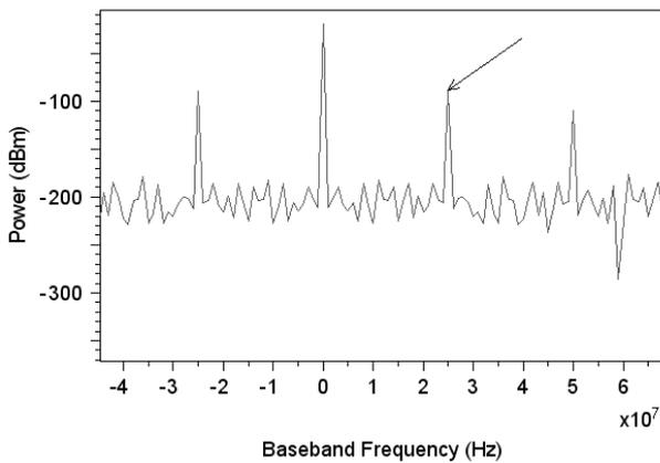
Fig. 1 RF Spectra of two tone directly modulated, CSO distortion at 25 MHz.
