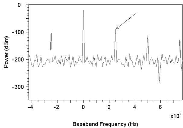
Fig. 4 RF Spectra of two tone externally modulated, CSO distortion at 25 MHz.
