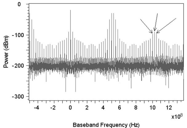
Fig. 5 RF Spectra of two tone directly modulated; CSO distortion at 1025 MHz, IMD at 1000 MHz & 1050 MHz.
