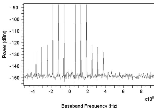
Fig. 6 RF Spectra of to three frequencies directly modulated.
