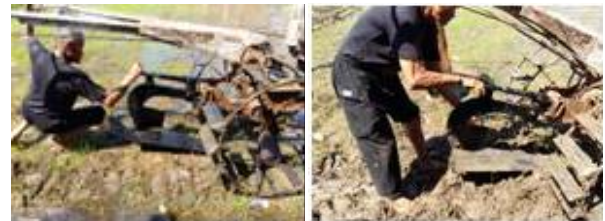
Fig. 3 Setting up the symmetric plough on a handtractor.
