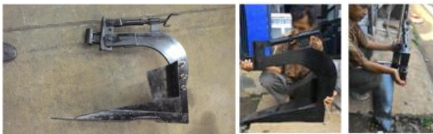
Fig. 2 The symmetric plough of 30° tilt angle at large.
