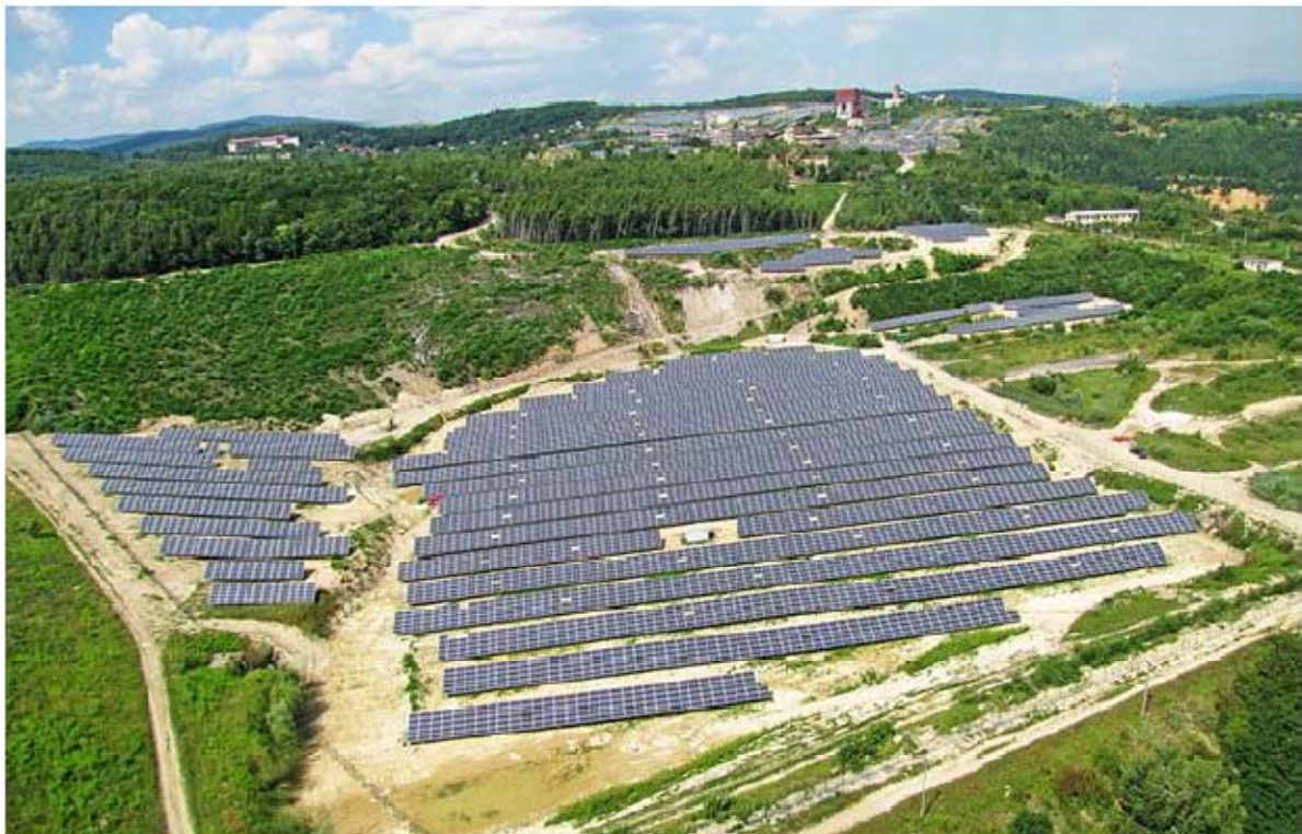
Fig. 13 The subsidence Košice-Bankov after reclamation; panoramic view – year: 2015. Solar panels: on a site of the former mining dumps; Afforestation (in the background): on a site of the former mining subsidence.
