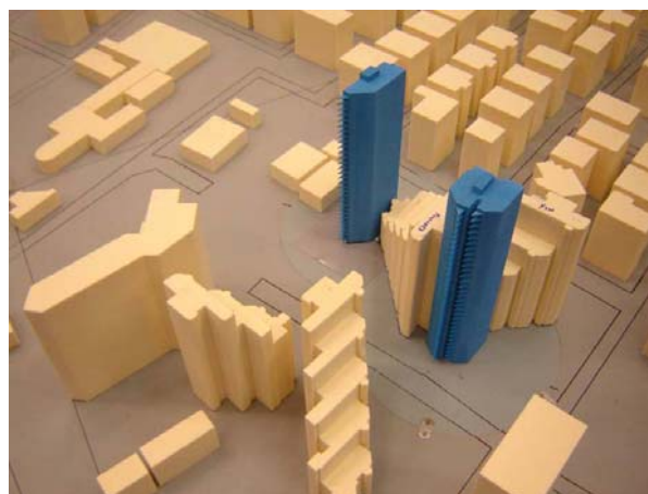
Fig. 5 Wind tunnel test model for the proposed towers with the surrounding buildings.
