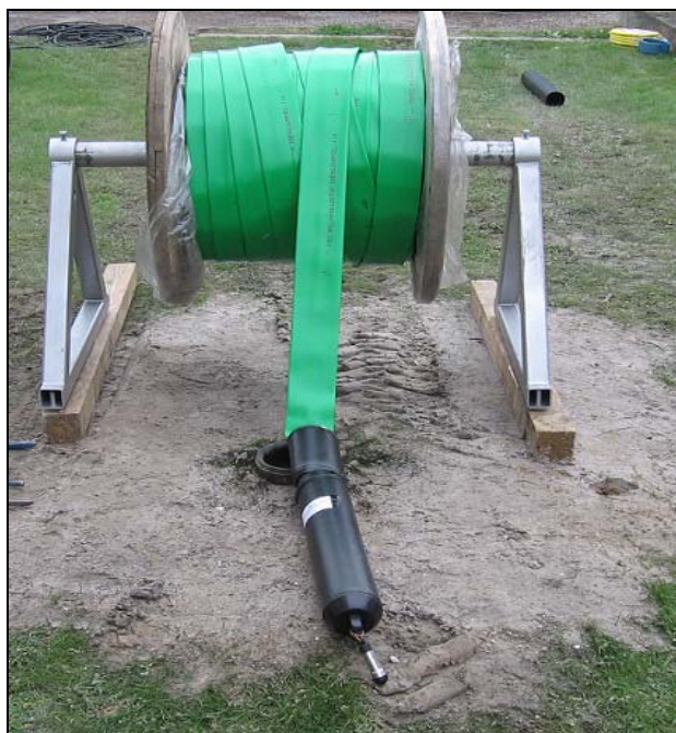
Fig. 7 The capsule comes to the site folded and is easily installed in the borehole by help of a bottom weight.
