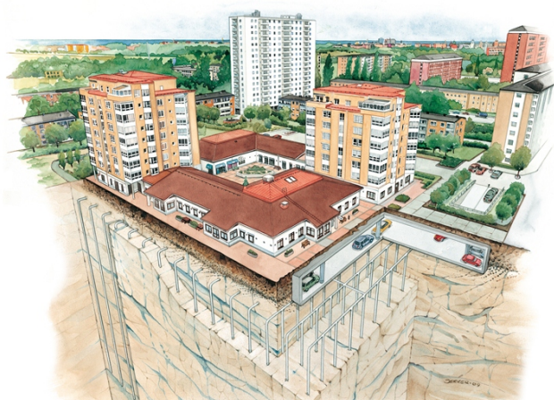
Fig. 3 The principle of BTES, a closed loop concept, where heat and cold are seasonally stored in a solid rock mass through a large number of densely spaced boreholes.
