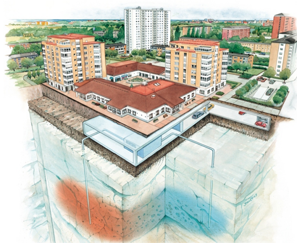
Fig. 1 The principal of ATES, an open loop concept, where heat and cold are seasonally stored in an aquifer.
