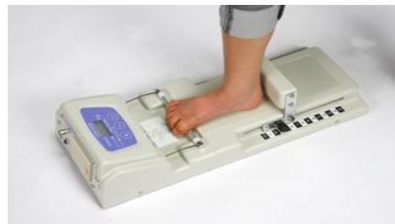
Fig. 1 Toe grip strength dynamometer (T.K.K.3360).
