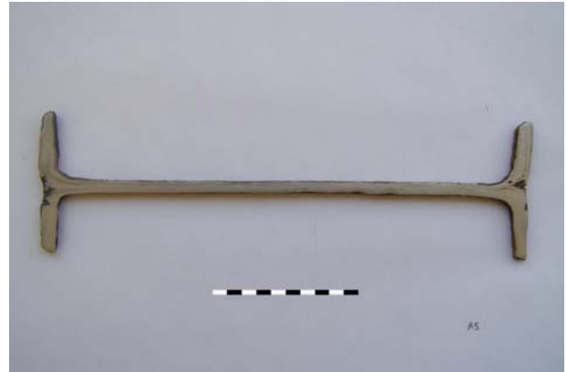
Fig. 13 A double tee clamp from the temple of Epikourios Apollo, without any welding in the middle.
