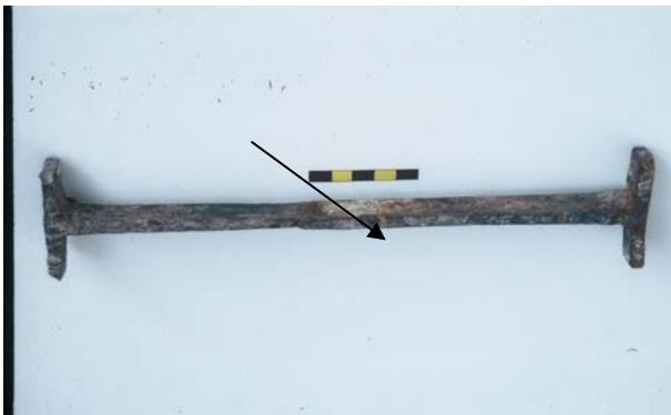
Fig. 4 An arrow shows a white spot, which indicates the hot welding point (1,200 °C) between two simple clamps into one double tee clamp.
