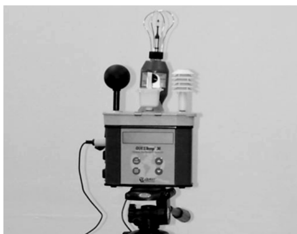
Fig. 5 Thermal stress monitor QUESTemp° 36.
