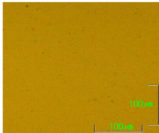
Fig. 4 Microstructure of polymer-rubber modified bitumen (CR) after 180 °C temperature conditioning measured on the bottom of cylinder after 7 days.
