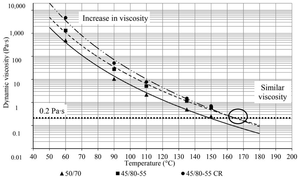
Fig. 1 Dynamic viscosity vs. temperature.
