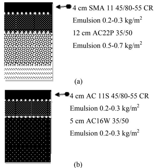
**Fig. 5 Trial sections containing polymer-rubber modified bitumen 45/80-55 CR: (a) wearing course SMA 11; (b) wearing course asphalt concrete AC 11.**
