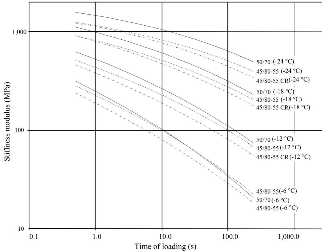
**Fig. 2 Stiffness modulus isotherms vs. time loading for non-aged binders at low temperature.**
