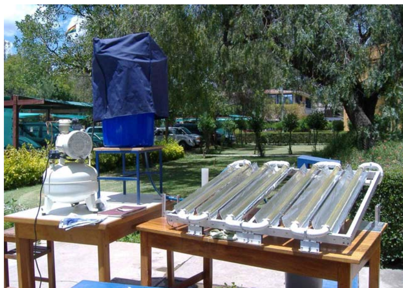
Fig. 7 Continuous flow solar concentrator.
