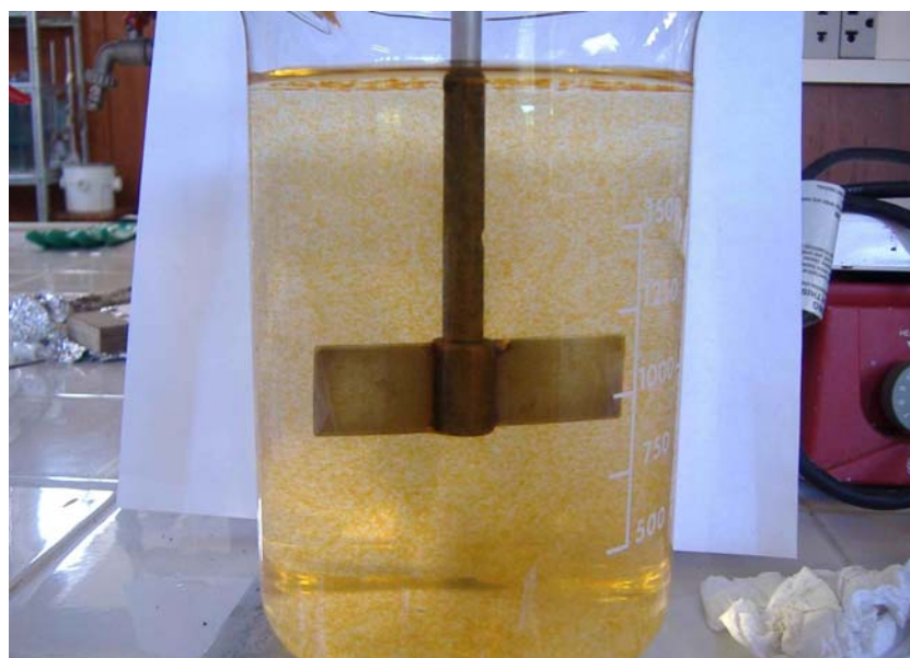
Fig. 9 Flocculation (Willcomb Index = 6-8) under controlled agitation (shear rate = 33\text{ s}^{-1} ). Spiked groundwater (1,000 μg-As(V)/L).
