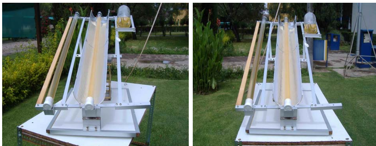
Fig. 5 Experimental apparatus tracking sun position during irradiation.
