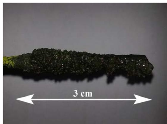
Fig. 2 W-cathode photograph after electrolysis in molten  $\text{NaCl-KCl-CrF}_3-\text{K}_2\text{SiF}_6$ ;  $i = 0.27 \text{ A}\cdot\text{cm}^{-2}$  at 850 °C.
