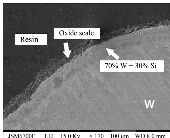
**Fig. 5** SEM micrograph of the cathode cross section after electrolysis of molten  $\text{NaCl-KCl}_{\text{eq.}}\text{-CrF}_3\text{-K}_2\text{SiF}_6$  system with  $i = 0.27 \text{ A}\cdot\text{cm}^{-2}$  at  $850\text{ }^{\circ}\text{C}$  during 1 h.
