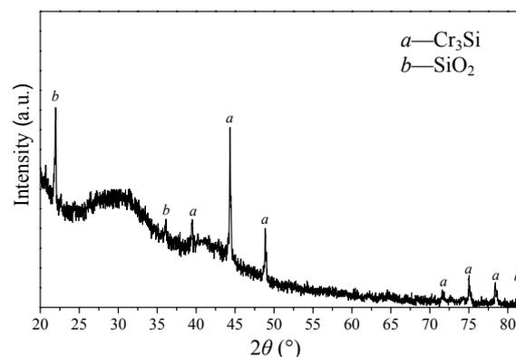
Fig. 3 XRD (X-ray diffraction) pattern of the cathodic product electrolyzed for 1 h.
