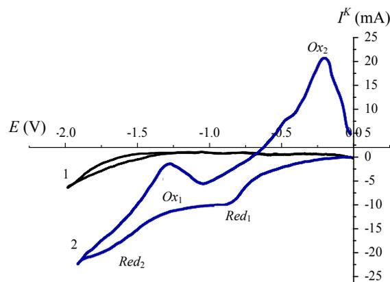
Fig. 1 Cyclic voltammograms of the  $\text{NaCl-KCl}_{\text{eq.}}-\text{CrF}_3-\text{K}_2\text{SiF}_6$  system at 850 °C; cathode—Pt,  $v = 0.1 \text{ V}\cdot\text{s}^{-1}$ : 1— $\text{NaCl-KCl}_{\text{eq.}}$ , 2— $\text{NaCl-KCl}_{\text{eq.}}-\text{CrF}_3$  ( $1 \times 10^{-5} \text{ mol}\cdot\text{cm}^{-3}$ )- $\text{K}_2\text{SiF}_6$  ( $2 \times 10^{-5} \text{ mol}\cdot\text{cm}^{-3}$ ).
