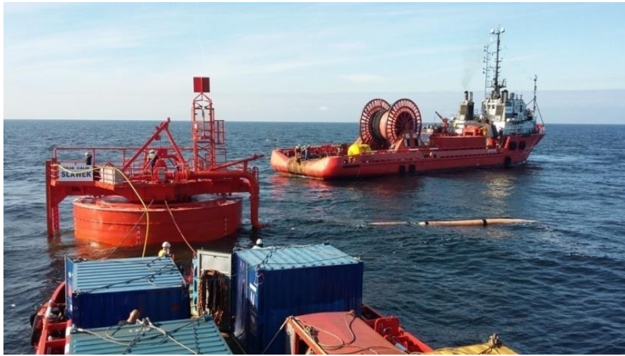
Fig. 3 Maintenance off-shore infrastructure - Catenary Anchor Leg Mooring CALM buoy by the AHTS vessels Source: Own study.
