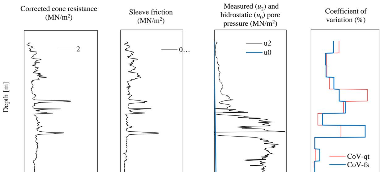
Fig. 2 Measurements of basic parameters and calculation of CoV for CPTu2.
