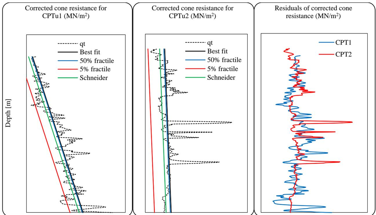
**Fig. 5** Characteristic values of corrected cone resistance for CPTu1 and CPTu2 and respective residuals.
