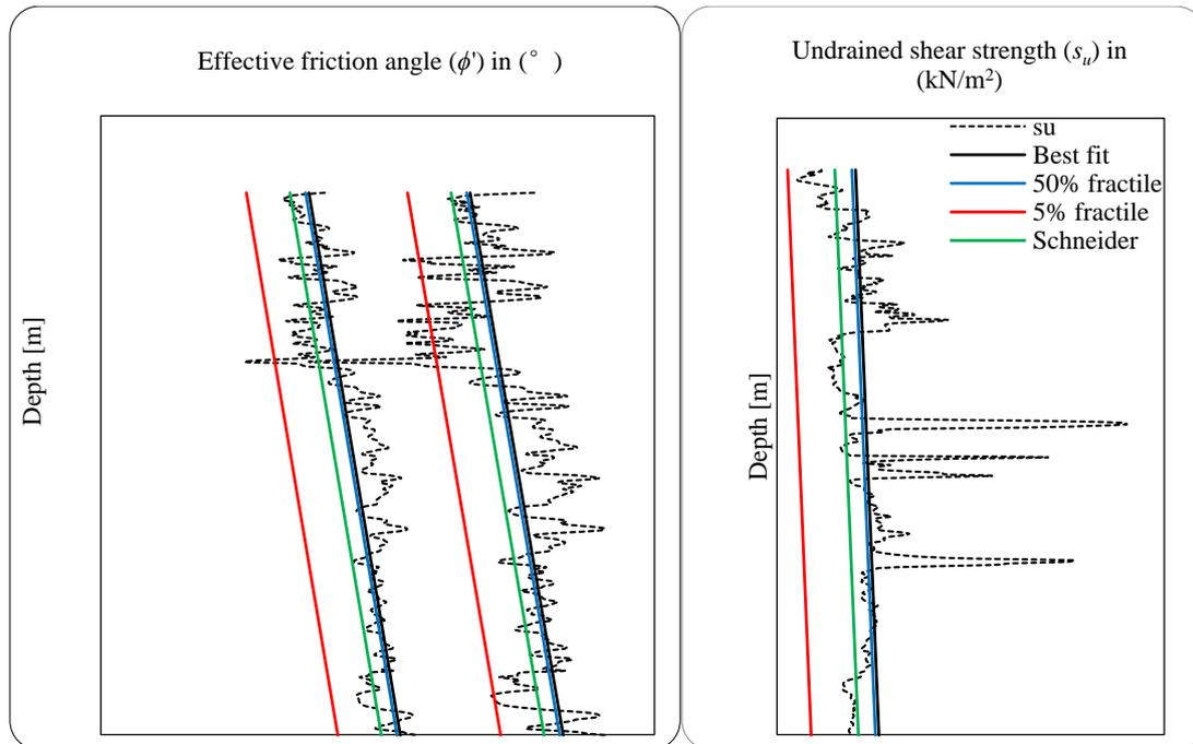
**Fig. 8** Characteristic values of effective friction angle and undrained shear strength.
