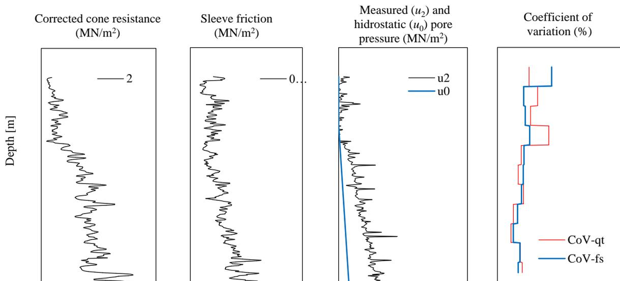
Fig. 1 Measurements of basic parameters and calculation of CoV (coefficient of variation) for CPTu1.
