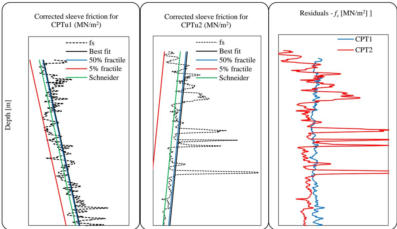
Fig. 6 Characteristic values of sleeve friction for CPTu1 and CPTu2 and respective residuals.
