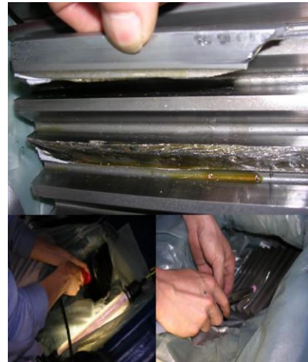
Fig. 7 Remove cracked teeth and grind.
