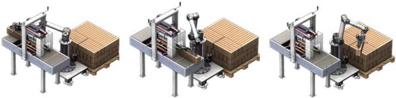
Fig. 5 Sequence of robot activities: scan, dispose in the sealing machine, remove and stack.
