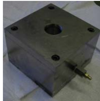
Fig. 1 Oil-hydraulic component to restrict pressure change owing to oil temperature change.
