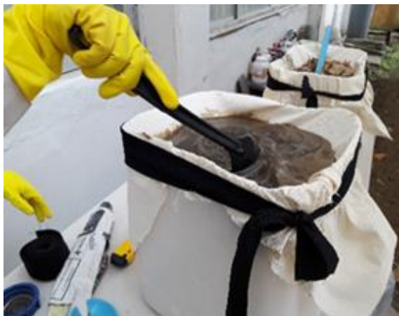
Fig. 2 Thickening of sludge.
