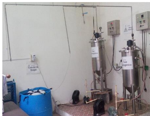
Fig. 1 Pilot plant of the anaerobic digester in phase.
