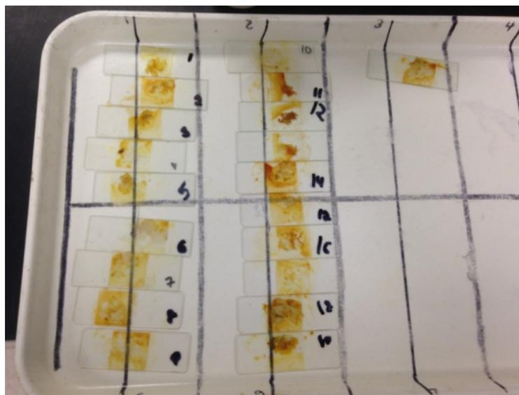
Fig. 6 Oyster tissue slides in pan numbered by oyster from which they were obtained.
