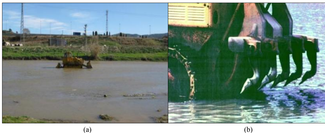
Fig. 9 (a) Tractor working in the Llobregat riverbed; (b) detail of tractor nails.
