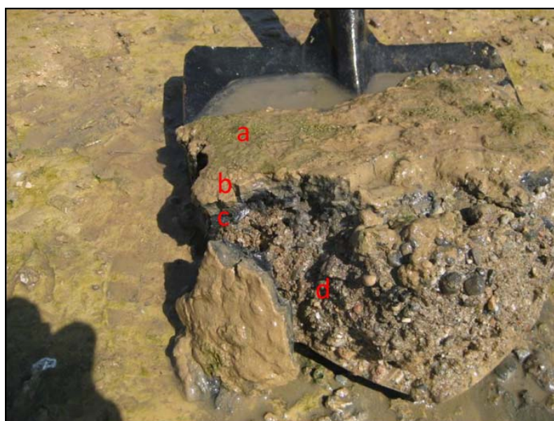
Fig. 10 Soil below the riverbed before scrapping. From top to bottom: (a) first layer with algae activity, (b) brown clay layer (oxic level), (c) grey clay layer (anoxic level), and (d) bottom high permeability gravels and sands. Below is the top of the aquifer, which receives the water leaking from the soil above.
