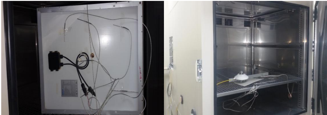
Fig. 1 On the right, a pictorial illustration of the solar panel inside the SEC 1100 chamber. On the left, the back of the solar panel and the temperature sensors fixed on it.
