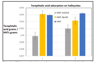
Fig. 4 This graph shows the grams of terephthalic acid absorbed by one gram of halloysite in solution.
