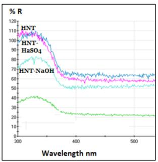
Fig. 3 In the diagram of diffuse reflectance the reflectance corresponding to haloisite can be observed without treatment and as it is radically reduced when using concentrated sulfuric acid treatment for 1 hour, treatment with 1 molar sulfuric acid for 1 hour and treated haloisite with sodium hydroxide.
