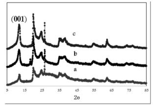
Fig. 2 The XRD spectra of halloysite: (c)halloysite treated with  $H_2SO_4$ , as well as(a) halloysite treated with NaOHand (b)free halloysite of treatmentare illustrated.
