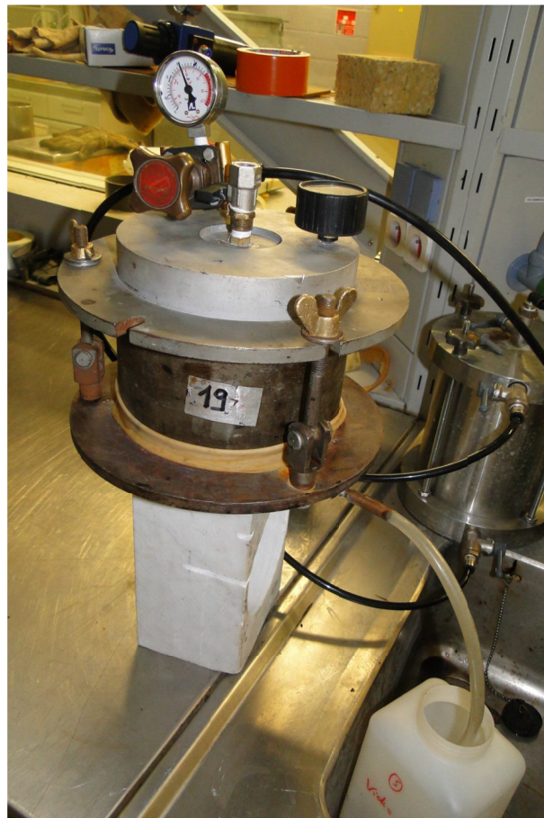
Fig. 3 Test equipment for measuring permeability of specimen.
