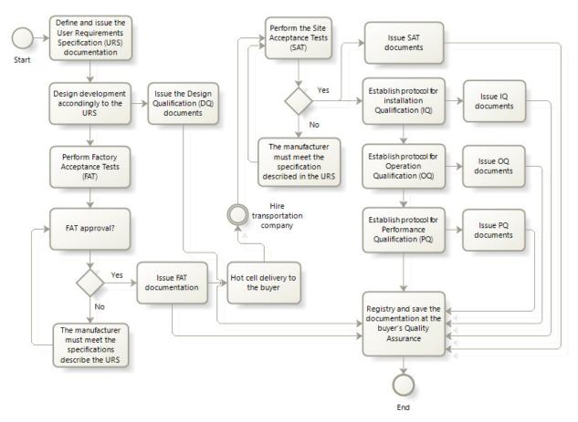
Fig. 1 Box-diagram for hot cell design, purchase and respective qualifications.
