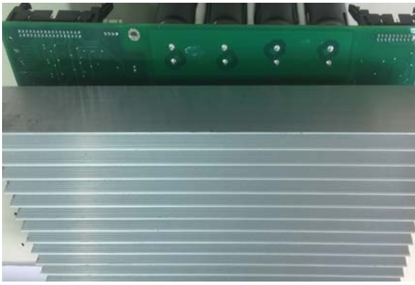
Fig. 24 Block of force circuit with heat radiator.
