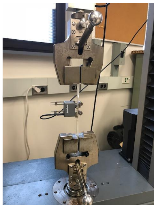
Fig. 2 The experimental set up for measuring the tensile modulus.
