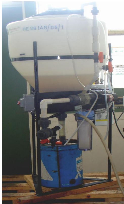
Figure 1. Biodiesel laboratory processor unit.
