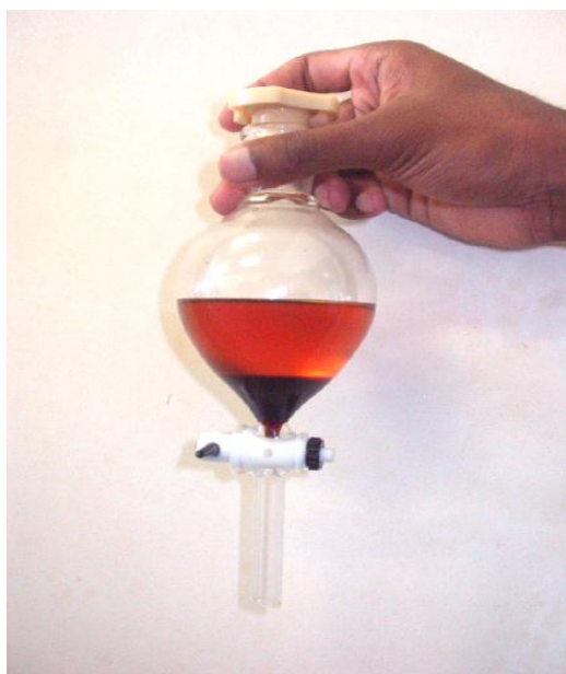
Figure 3. Flask with two distinct layers of biodiesel and glycerine.
