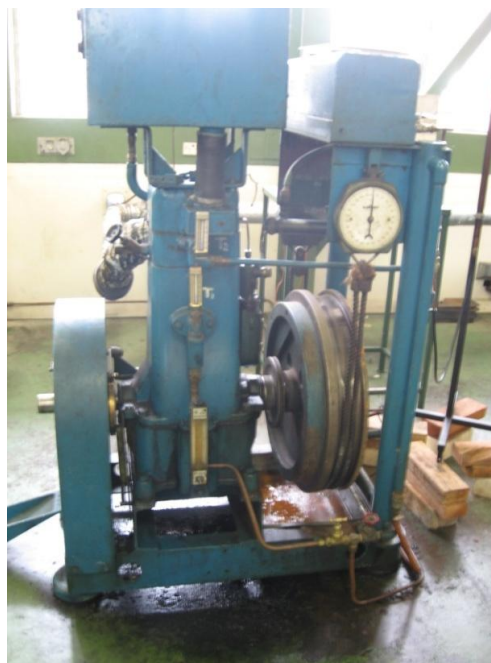
Figure 2. Fuel performance testing apparatus.
