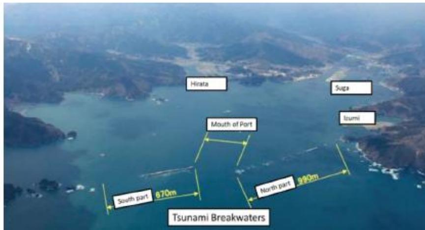
Fig. 26 Picture of Kamaishi Bay with partially collapsed breakwaters extracted from Ref. [22].
