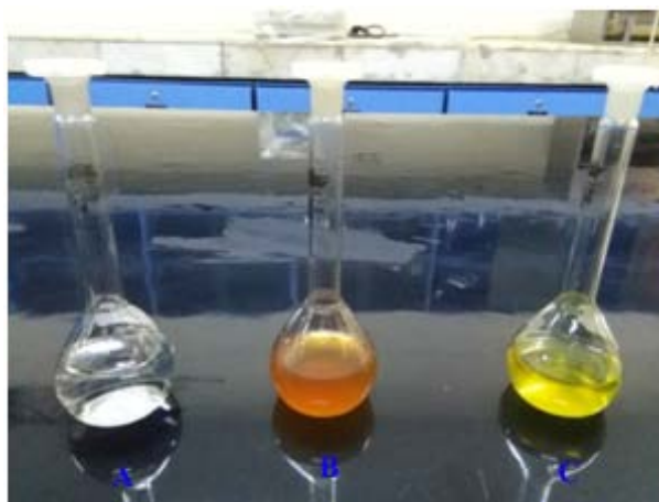
Fig. 3 Color changes observed before and after the formation of CuO NPs (A) \text{CuSO}_4 \cdot 5\text{H}_2\text{O} precursor, (B) leaf extract of Khat , and (C) CuO NPs.
