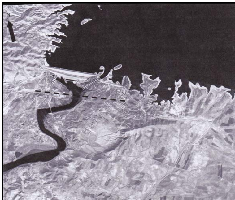
Fig. 23 Aerial view of the Dam area showing alignment of downstream sinkholes [9].
