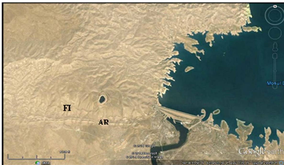
Fig. 5 Google Earth image of the Mosul Dam site, located within Butma east Anticline. AR = anticlinal ridge, FI = flat iron [5].
