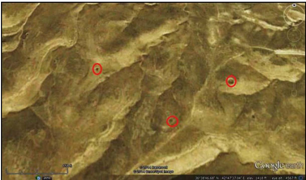
Fig. 9 Enlarged Google Earth image showing many sinkholes (dark spots encircled by red color), in the upstream area of the dam site [5].
