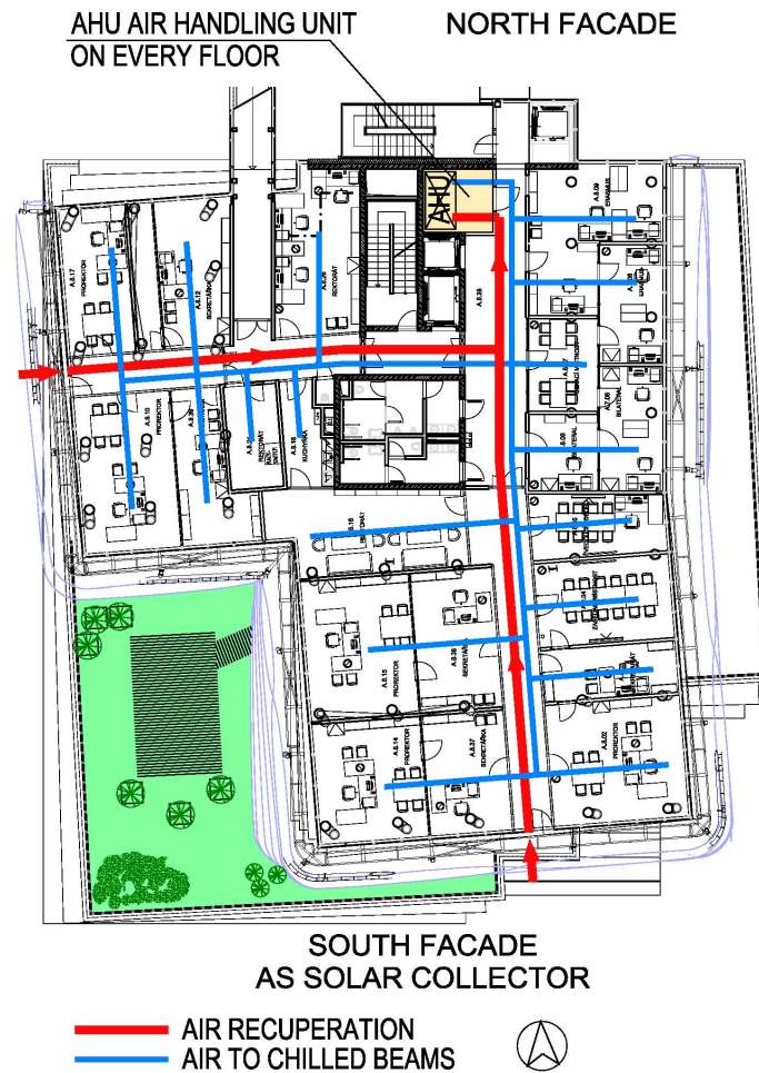
Fig. 10 Schema of recuperation and air distribution to chilled beams [3].
