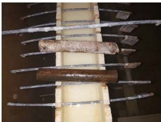
Fig. 4 Alternative coating salt mist test image with zinc phosphate coating.
