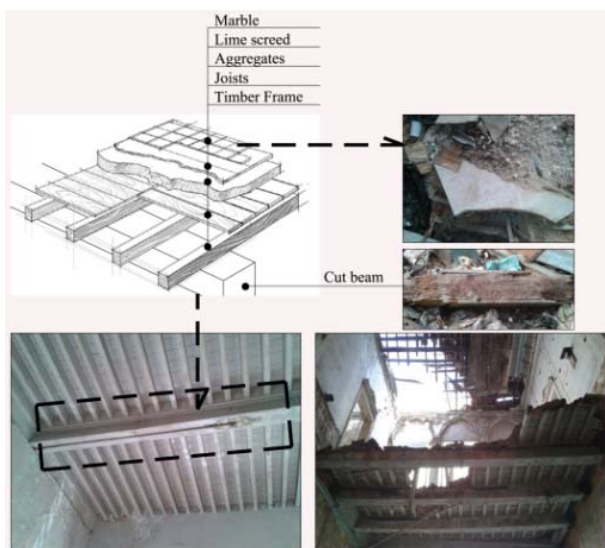
Fig. 19 Construction of intermediate ceiling in kaaki house before 1880s (idem).
