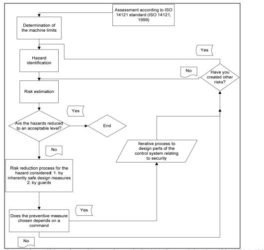
*Figure 3.* Strategy for certifying safety and support the standardization's framework based on ISO 13849-1 (ISO 13849-1, 2015).
